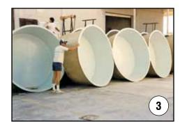
We manufacture one piece round tanks up to 8' 6" in diameter. Tanks over 8' 6" diameter are usually produced in two or more sections in order to be road legal, which saves on freight as it does not require a wide load permit. Round tanks are available with a flat or a tapered bottom. Most models over 4' deep require the installation of top jump rings to achieve the added height and require assembly.
